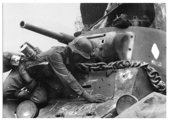
Soviet BT-7 cavalry tank, probably knocked-out by a antitank rifle
